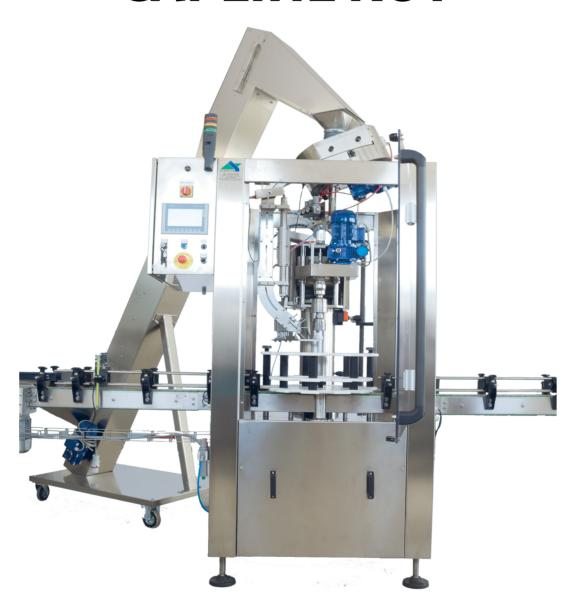
Single head capping machine Capline ROT is rotary indexing capping machine that has been designed for closing of various container types (made of plastic, glass and metal) with screw, press-on and pilfer proof caps. The cap is automatically oriented and applied on the bottle neck.
